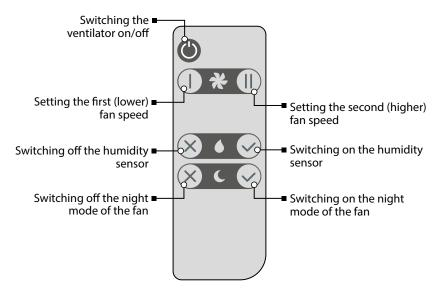
When switched on using the **On/Off** button on the remote control, the ventilator starts to operate at the speed at which it was switched off.
